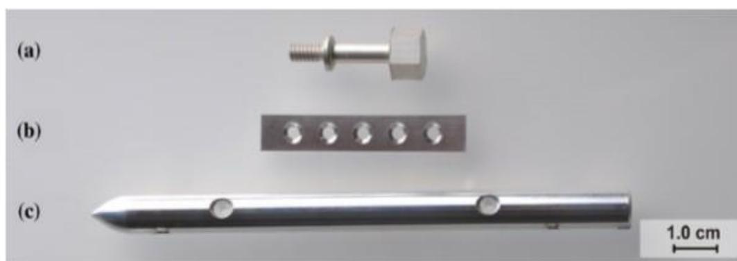
**Figure 1.** An Illustration of Various Orthopaedic Graft Geometries Made of Magnesium Alloys. (a) MgCa0.8 screw (b) ZEK100-plate (c) intramedullary LAE442-nail.<sup>9</sup>
